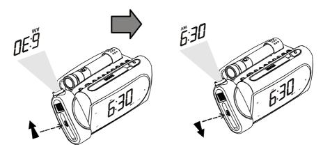
5.) If the image appears 'fuzzy' and out of focus, slowly rotate the **FOCUS** adjustment ring clockwise or counter-clockwise until you obtain the sharpest image.
